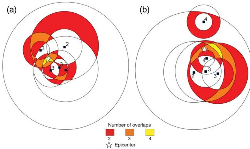
**Figure 2.** The criterion for the epicenter. Squares depict localities, and the numbers signify the corresponding intensities. Colors mark places where two, three, or four rings overlap. (a) The maximum number of overlapping rings is four, and the epicenter can be found in the area of overlap. (b) The maximum number of overlapping rings is four, but the epicenter does not coincide with the area constrained by the overlapping rings, producing a false solution.
