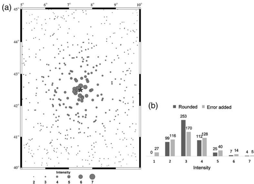
**Figure 3.** (a) A map of the 500 localities generated randomly and used to obtain samples of intensity data points (IDPs) randomly. The star demarks the fixed epicenter. (b) The numbers of synthetic intensities created for 500 localities. The dark columns depict the intensities that were rounded to the closest integer, and the light columns represent intensities containing errors.
