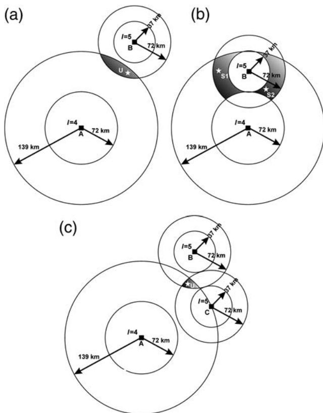
**Figure 1.** Epicenter determination for sparse sets of intensity data. The black squares demark localities A, B, and C with intensities 4, 5, and 5, respectively. The arrows show the lower and upper radii that encompass the localities that were computed using an intensity attenuation relationship. The shaded areas constrained by the overlapping rings contain all possible epicenters that produce the corresponding intensities, and their sizes correspond to the location uncertainty.
