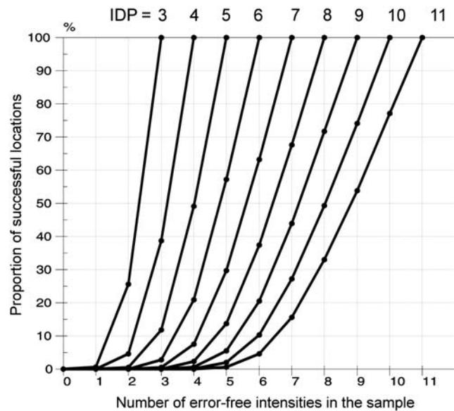
Figure 7. The proportion of successful locations (y axis) versus the number of error-free intensities in the sample (x axis). Successful is defined as when the true epicenter is found within the area of overlapping rings. The nine curves refer to samples with 3–11 IDPs.
