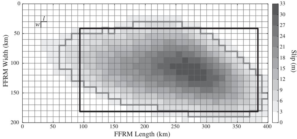
**Figure 1.** Schematic of fault trimming process. A synthetic finite-fault rupture model (FFRM) is plotted showing the slip for each subfault of length  $l$  and width  $w$ . The thick gray line bounds the maximum and minimum subfault indexes for each column  $i$  and row  $j$  for which the slip  $D_{ij} \geq D_{\text{lim}}$ . The thick black line represents the effective rupture dimensions used for  $L$  and  $W$ .
